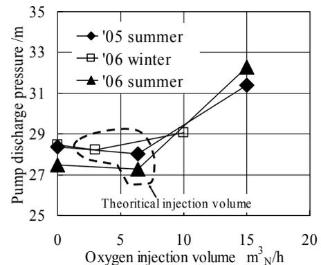
Figure 1 Pressure loss
