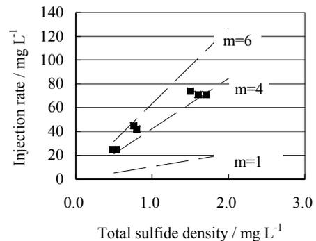
Figure 2 Empirical factor of polyferric sulfate adding
