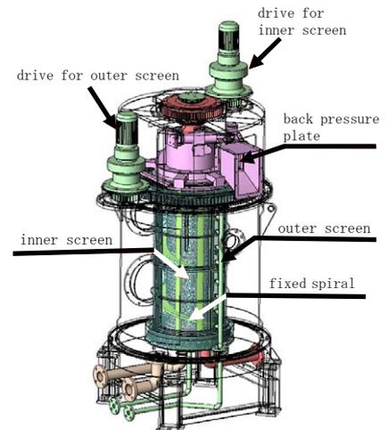
Figure 1 Schematic diagrams of DCFP
