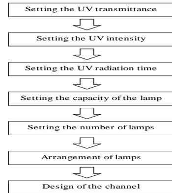
Fig.2 Design procedure for an open channel UV disinfection
