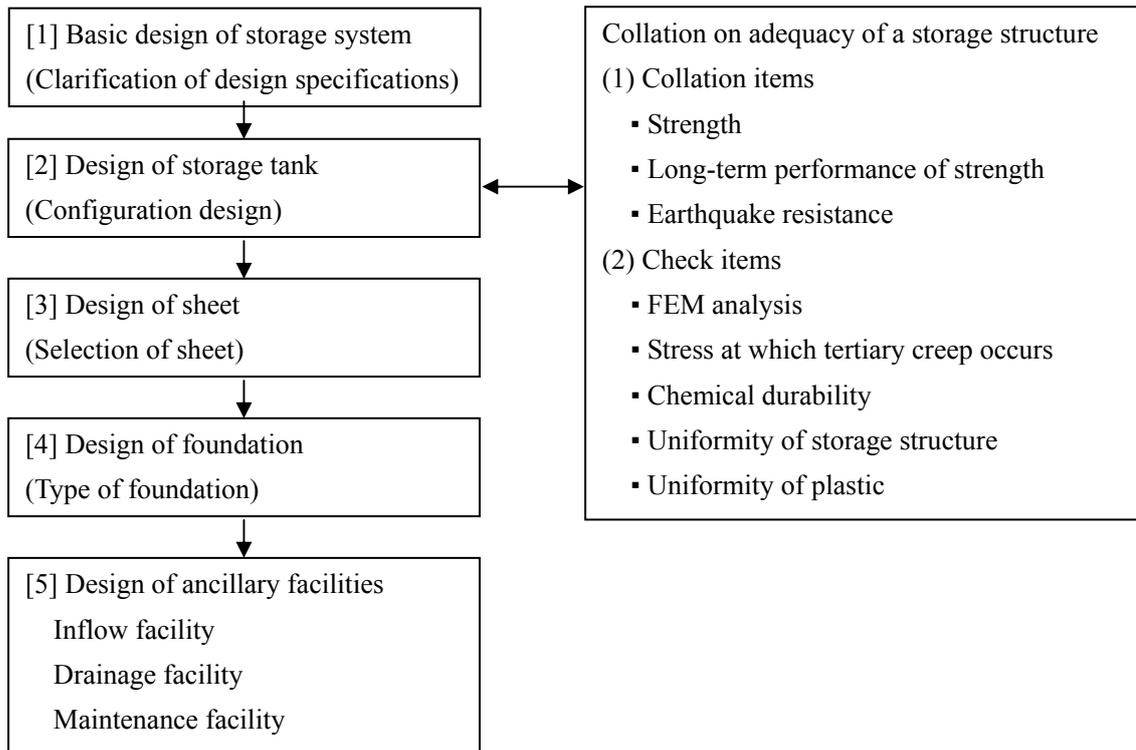
Figure 1 Plastic storage system design procedure
