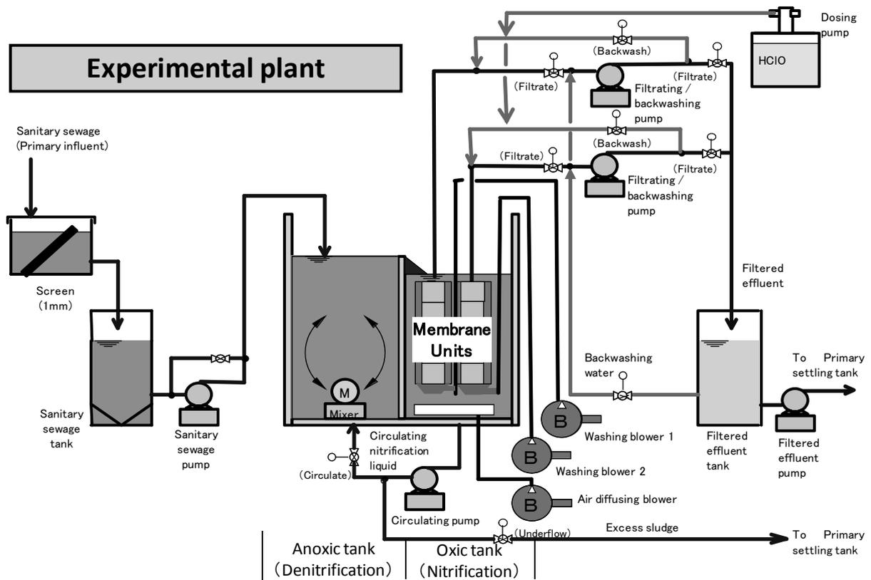
Figure 1: The flow chart of the MBR experimental plant that uses ceramic flat membranes.
