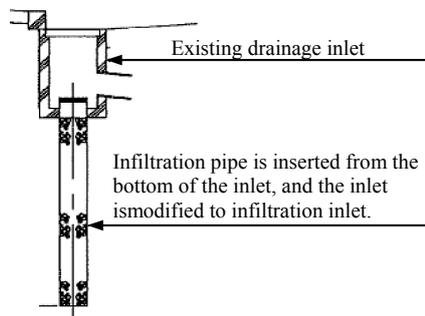
Figure-1 Infiltration facilities by modifying existing drainage inlets
