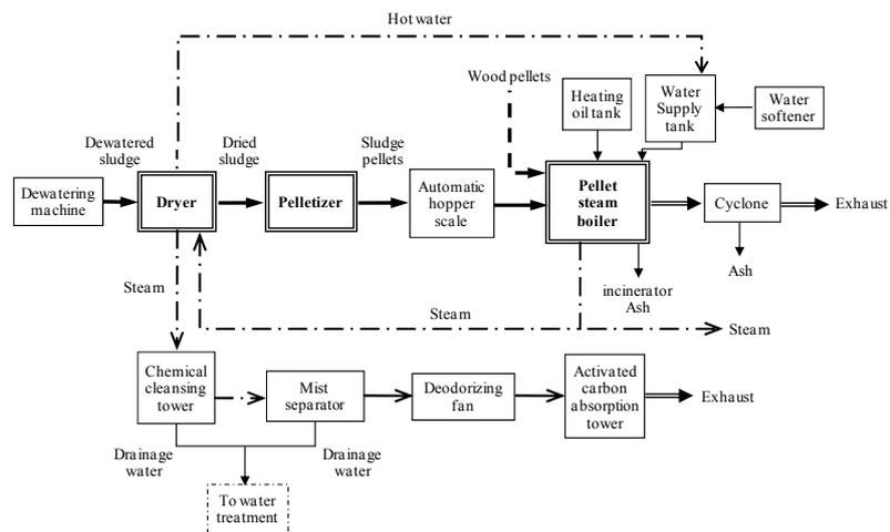
Figure 1. General Flow Chart of the Demonstration Facility
