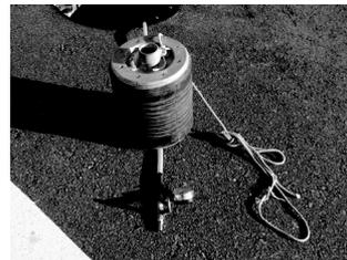
Cut-off plug used to stop water flow and store enough water to create flow speed needed when flushing.
