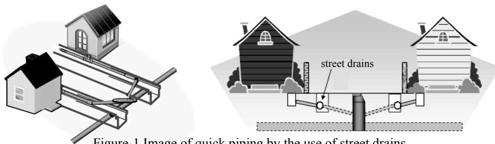
Figure-1 Image of quick piping by the use of street drains
