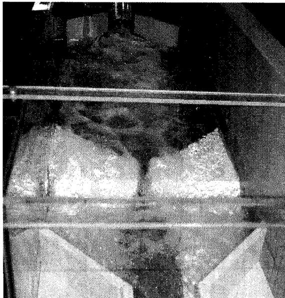
跳水状況 ( $Q=0.048\text{m}^3/\text{S}$ )
