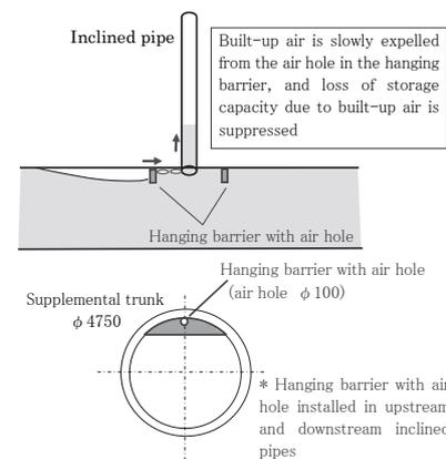
**Figure 2: Overview of hanging barriers with air holes**
